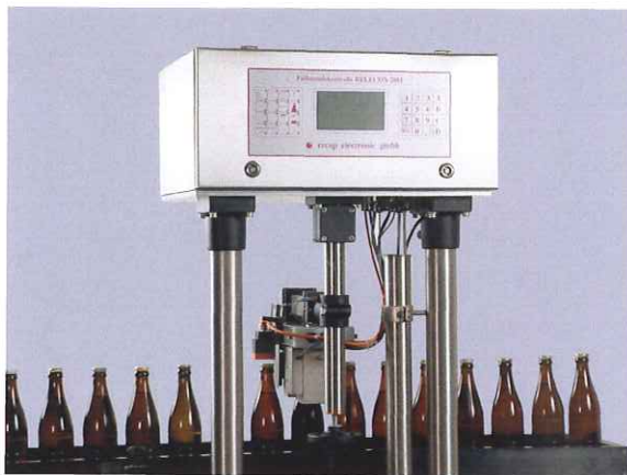
HF-fill level inspection '201'
